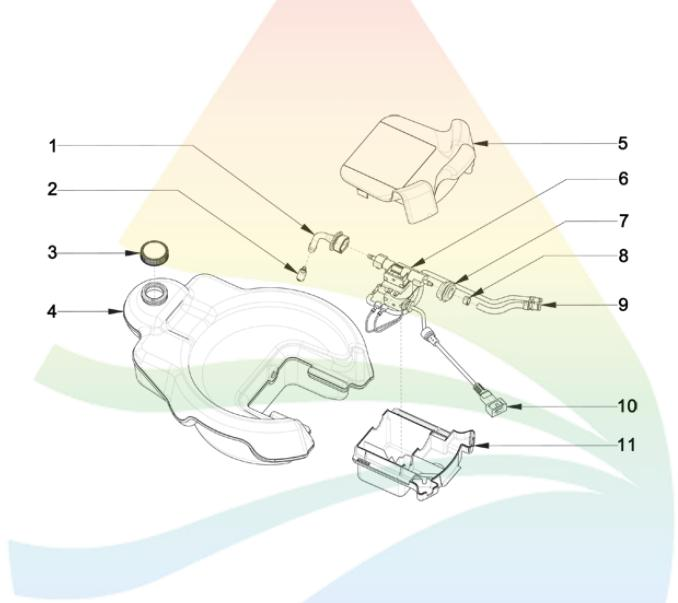
This category covers the complete AquaMate II (AM-2) pump assembly that includes the water pump, electric cord, and pump housing.
