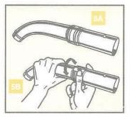
Adjust airflow control sleeve on top of curved wand. Close opening with airflow control sleeve for full power.
