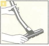
CONNECTING WAND TO FLOOR AND WALL BRUSH: Insert the end of the curved metal wand into the floor and wall brush. Align the button lock on the wand with the guide on the brush collar. Slide the button into the guide to engage the lock.
