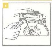
screwdriver, Using a remove the panel from the back of the machine by pressing up on the two latches on the underside of the rear panel. Move the bottom of the rear panel towards you, lifting up.
