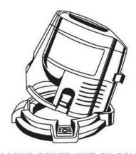
PLACING POWER UNIT ON DOLLY: Place power unit on dolly by tipping front end slightly upward so that the lip at the back of the unit slips under the lip at the rear of the dolly. Unit will then drop into place on the dolly. A foot latch at the front of the power unit locks unit in place. To remove, depress foot latch and lift unit from dolly by tipping slightly backward and pulling upward.
