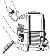
**SPRAYER ASSEMBLY:** The Rainbow Sprayer Assembly attaches to your Rainbow wands and is used to spray insecticides, moth-proofing solutions, etc. It can also be used with liquid fertilizers or plain water on your houseplants. To use the Sprayer, simply fit it onto your Rainbow curved wand handle and connect the hose to the air exhaust on your Rainbow.
