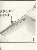
Connect the Straight Wand and Handle (Short Curved Wand) and insert into the Bottom Wand with Tool on end.
