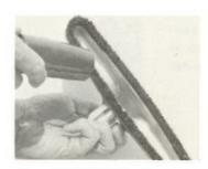
Dust and gritty dirt from cracks and crevices must be removed from floors to prevent scratching and keep them attractively clean. Use full suction as you glide Tool over floor. Tool will pick up surface litter and dirt from cracks and crevices.
