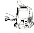
4 ENERGIZING THE POWER NOZZLE: With the electrical connections made, the power unit master switch will energize both the power unit and the Power Nozzle. However, the power unit will not activate the power nozzle brush roll. The switch actuator in the Rainbow handle must be actuated to operate the Power Nozzle. To remove the electrified hose from the power unit, squeeze coupling side latches and pull hose from intake opening.
